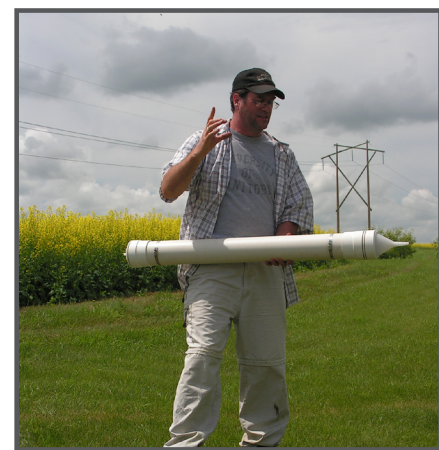
Dr. David Lobb explains his sediment sourcing research using suspended sediment collectors (pictured) and radionuclides at a field tour of the South Tobacco Creek Watershed
